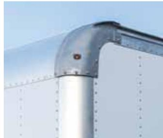
**Heavy-duty cast aluminum upper corner caps** also offer superior impact resistance. These proprietary caps add structural integrity to our front assembly; they don't just cover the hole. The ITB Industrial caps also overlap all mating surfaces making replacement easy and fast.
